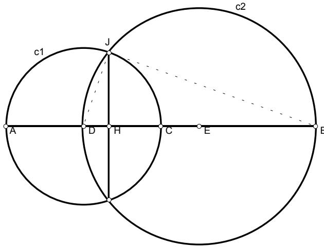
*Geometric Proof of Construction:* Use the notation in the diagram above and additionally label one of the points of intersection of the two circles **J**. Then triangles **DJB** and **DHJ** are similar right triangles. Thus,  $\mathbf{DH/DA = DH/DJ = DJ/DB = DA/DB = 1/3}$ . Notice also that  $\mathbf{DA/AB = 1/4}$ , by construction of **D**. If **DH** is taken as the unit length, then **DA = 3**, **AB = 12** and **AH = 4** whereby **AH/AB = 1/3** as desired.  $\square$
